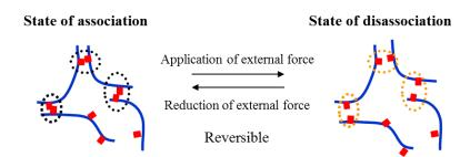
The viscosity of inorganic materials can be controlled with the addition of the polymer, and with this ability to control the viscosity, the polymer shows promise for uses as a viscosity modifier for electronics, construction, paints, and other areas.
